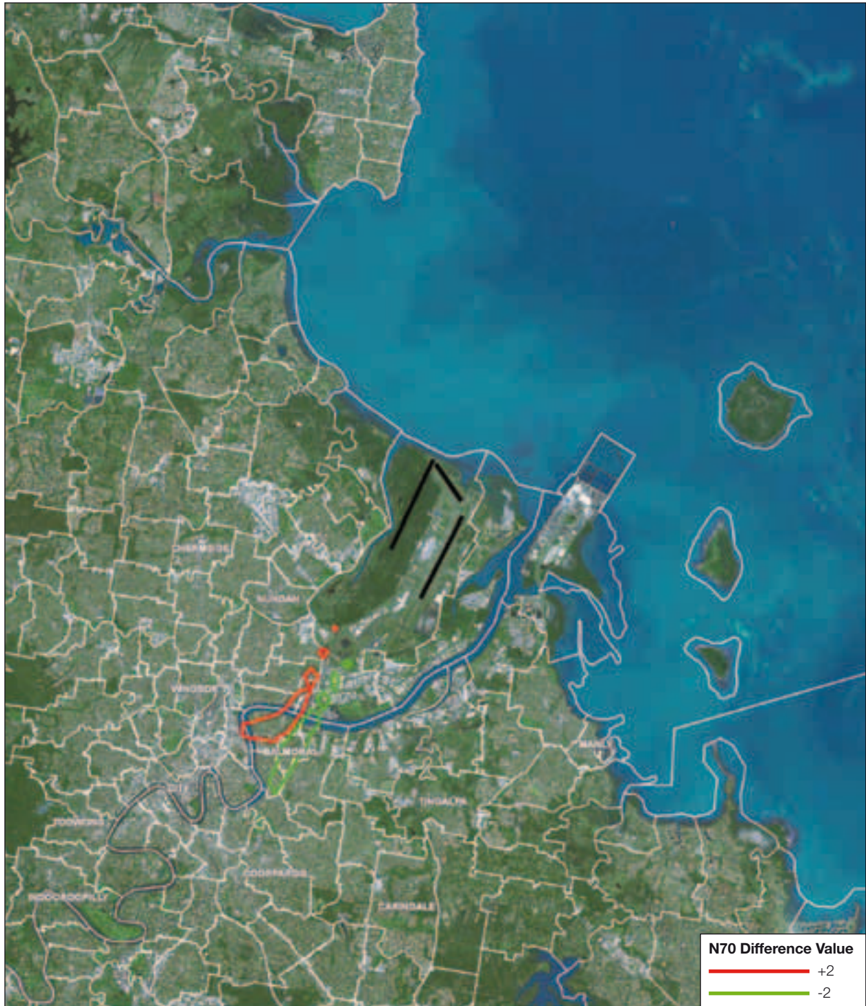
Figure 5.2f: Difference in N70 Overflights Between Option 1 and Option 2A Approach Tracks – Summer Weekday Day.
